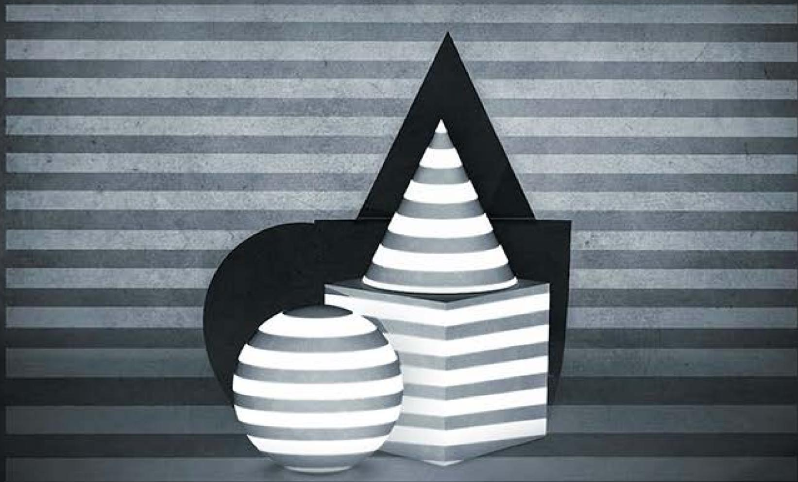
Scanner tool projecting a set of horizontal and vertical lines to calculate the accurate geometry for precise projection mapping.
